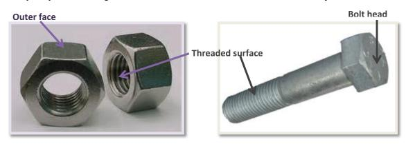
The average measured coating thicknesses in **each reference area** should be equal to or greater than the appropriate "local coating thickness" value in <u>Table 4</u>. AND
