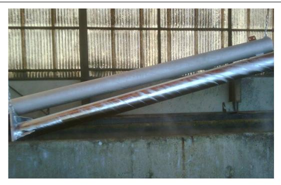
**Figure 2:** Two posts with different steel compositions after being galvanized at the same time. The top post is typical of steel from Categories C & D while the bottom appearance is typical of steel from Categories X & A. Both products comply with AS/NZS 4680.
