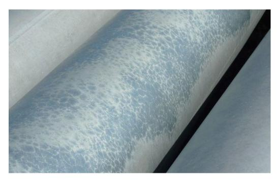
**Figure 3:** This galvanized pipe's steel composition is likely to be in Category B, shown by the scale-like appearance of the coating, where some on the Fe/Zn alloy has extended through to the surface. This product complies with AS/NZS 4680. Over time, the surface will change to a more even dull grey finish.
