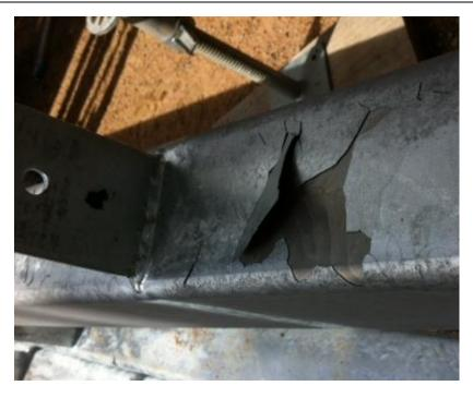
**Figure 6:** Category D steels are most likely to produce a galvanized coating where thick, brittle Fe/Zn alloy layers are formed and flaking occurs due to the excessive coating thickness. This article will not meet the requirements of AS/NZS 4680 due to the excessive flaking and should be rejected.
