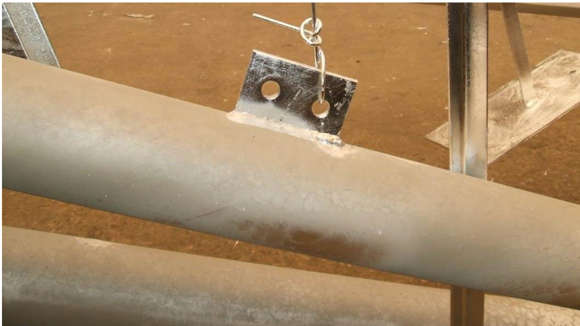
Figure 2: The majority of the pipe has a matte grey appearance, most likely due to the steel chemistry.
