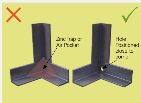
Figure 23: Inward Facing Angles – Venting Required
