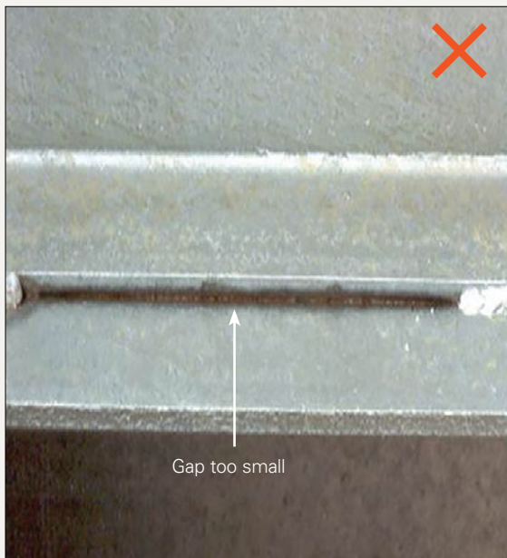
Figure 33: Overlapping Areas - Venting Unsatisfactory
