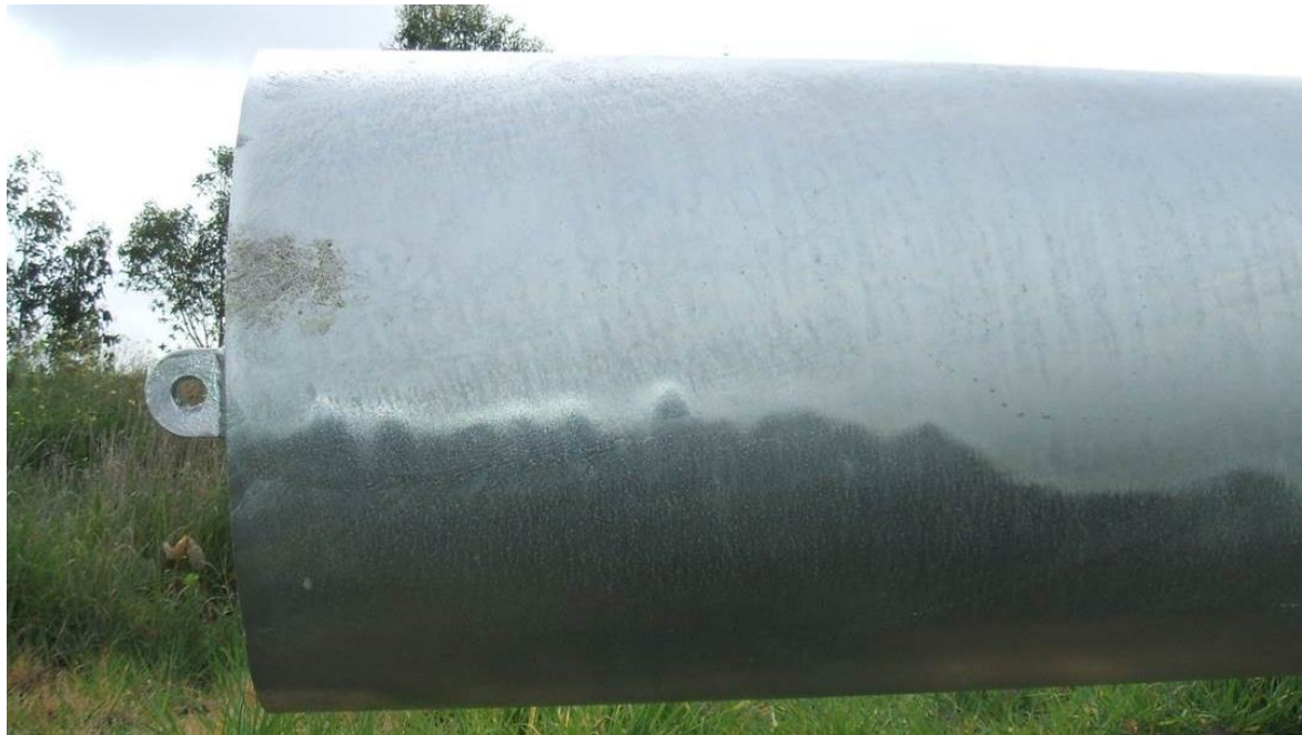
Figure 6: The duller section of the pipe has been exposed to the bath temperature for longer, with the shiny section consisting of pure zinc.
