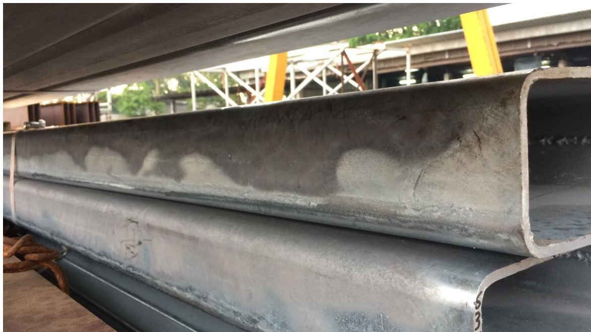
Figure 5: A well-defined barrier between shiny and dull sections could be a result of prolonged bath temperature exposure or the zinc cooling and losing fluidity during run off.
