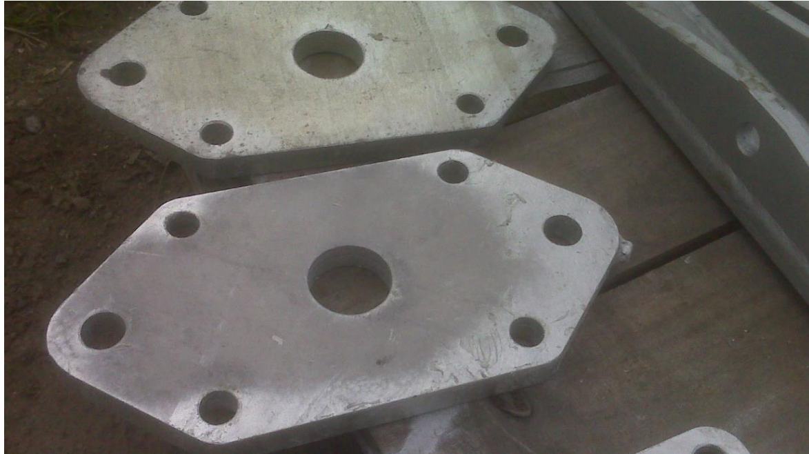
Figure 2: The thicker plate has cooled more slowly in the centre, causing a dull grey finish where alloy layers have grown to the surface.
