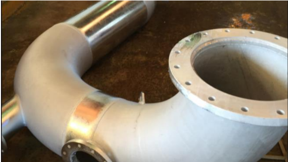
Figure 8: Steels with different chemical compositions on the straight and curved sections have been used, resulting in the straight sections being shiny and the curved sections dull.
