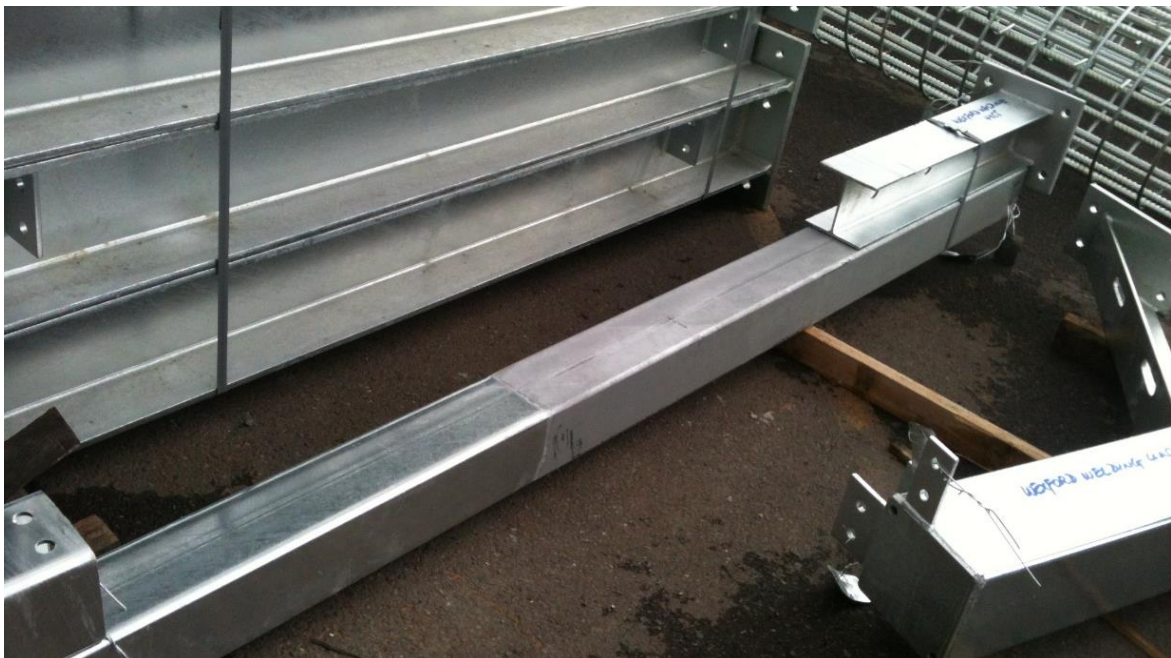
Figure 9: Steels of different compositions have been welded together in a straight square hollow section, resulting the differing appearance.
