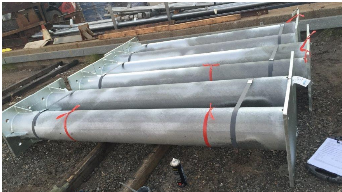
Figure 7: A small shiny section can be seen in the bottom right of the image, likely caused by the surface cooling at a different rate.
