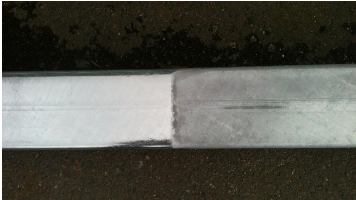
Figure 10: A close up of steel of different compositions being joined in a square hollow section, which is acceptable as long as the coating is sufficiently adherent.
