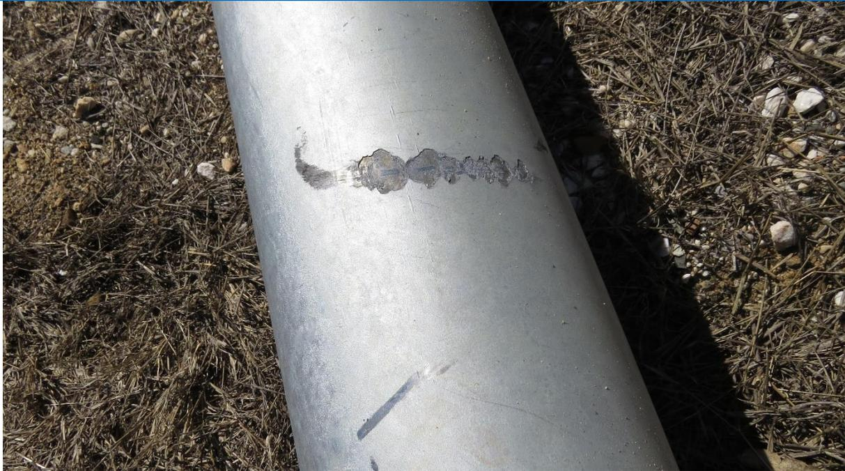
**Figure 7:** Impact during handling has caused flaking of the thick, brittle galvanized coating.
