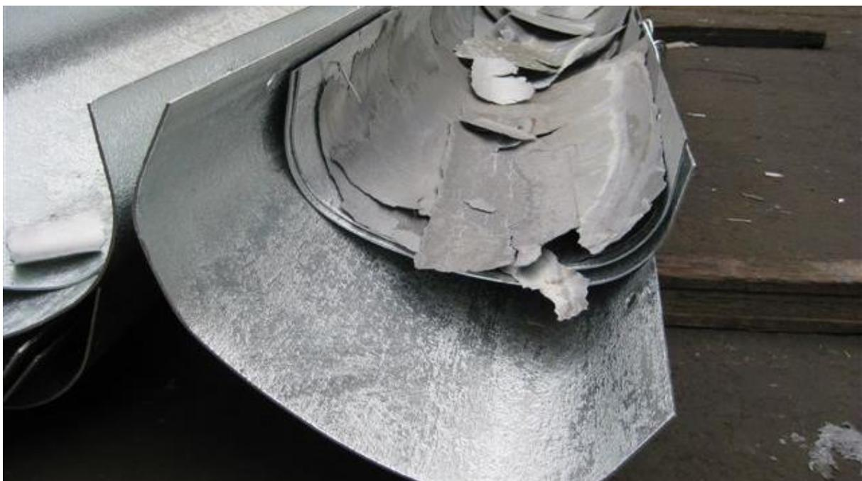
**Figure 4:** The galvanized coating is flaking off thin steel sheets. Thin steels should be cooled as quickly as possible after galvanizing in an attempt to prevent flaking
