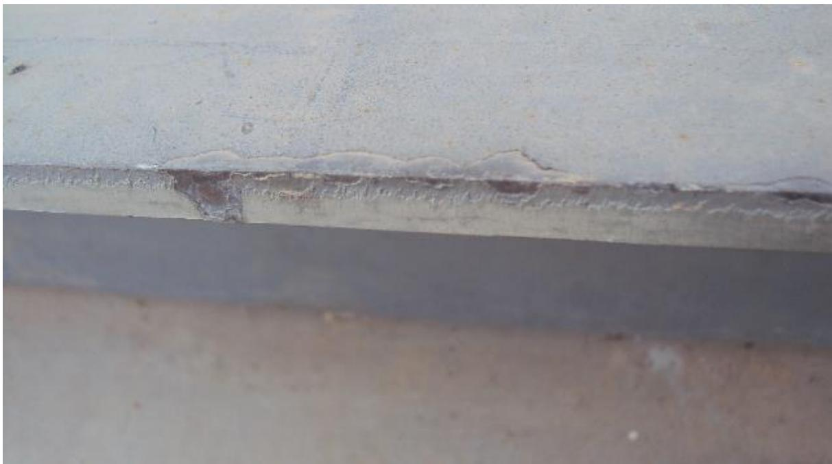
**Figure 6:** Handling damage has caused flaking near the edge of the galvanized article.
