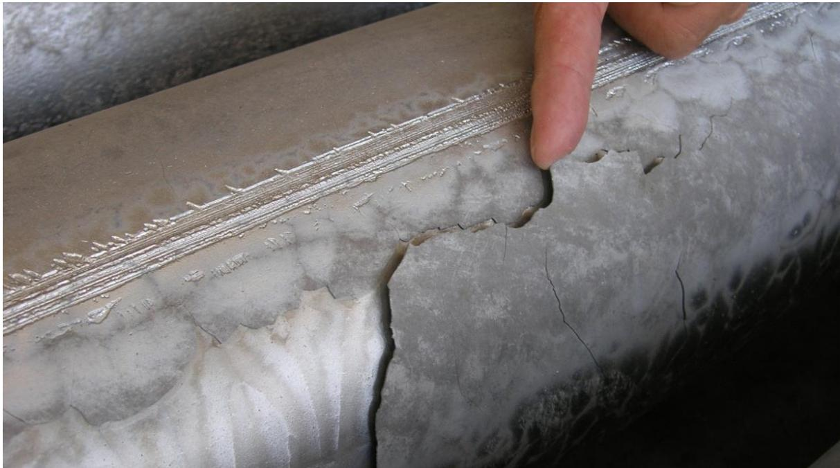
**Figure 3:** The zinc coating is flaking off a fabricated pipe due to the steel chemistry. The mottled grey appearance is indicative of a silicon content between 0.04% and 0.14% (see *TN Mottled Appearance*).
