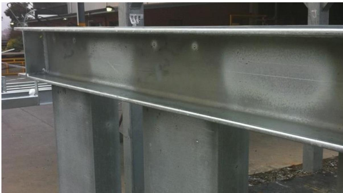
**Figure 3:** A dark grey coating is seen where steel is held at a higher temperature for longer and alloy layers can continue to form. More examples of both shiny and dull regions on the same article can be found in *Differing Appearance*.
