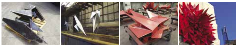
Figure 3: The Moment by Damian Vick, showing the four key stages of fabrication, galvanizing, painting and the final structure in place. This aesthetic sculpture is an example of a complex shape with sharp edges and is therefore perfectly suited to a duplex coating.
