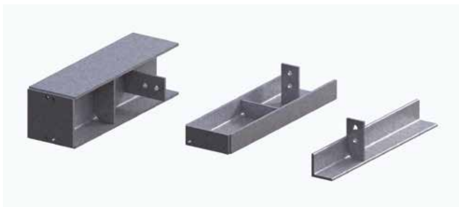
Figure 4: Illustrations in Appendix A of AS/NZS 2312.2 allow the designer to improve zinc flow in the HDG process, which will improve the aesthetics of the finished product, reduce the cost and eliminate danger to the galvanizing plant operators.
