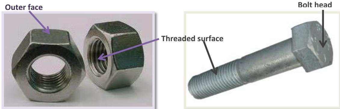
The *average measured coating thicknesses* in **each reference area** should be equal to or greater than the appropriate **“local coating thickness”** value in Table 4. **AND**
