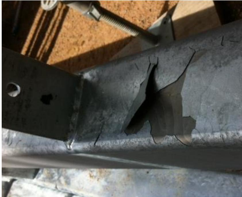
**Figure 6:** Category D steels are most likely to produce a galvanized coating where thick, brittle Fe/Zn alloy layers are formed and flaking occurs due to the excessive coating thickness. This article will not meet the requirements of AS/NZS 4680 due to the excessive flaking and should be rejected.
