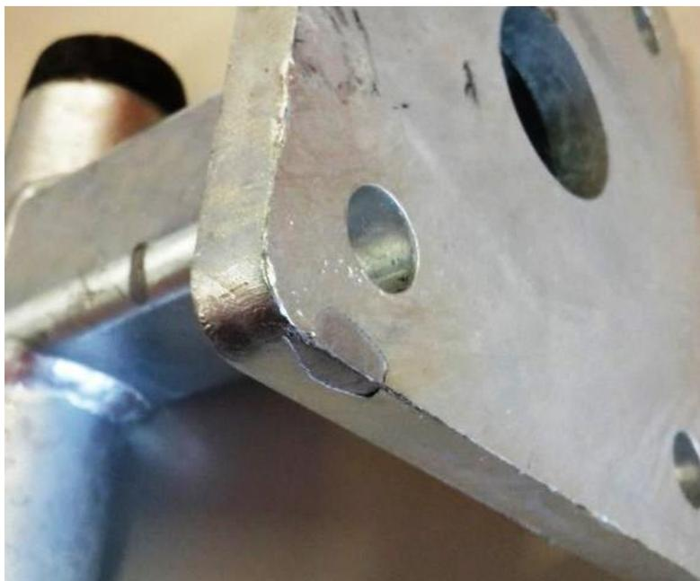
**Figure 5:** Handling has caused some damage to the edge of this thick galvanized coating, where some of the coating has been chipped. Thick coatings can result when steels from Categories C & D are galvanized. It is likely the coating will still meet the thickness requirements of AS/NZS 4680, and is acceptable, so long as the remaining product firmly adheres to the substrate.
