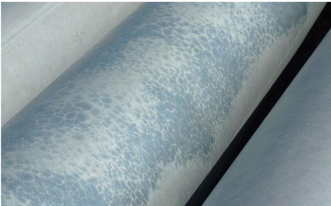
**Figure 3:** This galvanized pipe's steel composition is likely to be in Category B, shown by the scale-like appearance of the coating, where some on the Fe/Zn alloy has extended through to the surface. This product complies with AS/NZS 4680. Over time, the surface will change to a more even dull grey finish.
