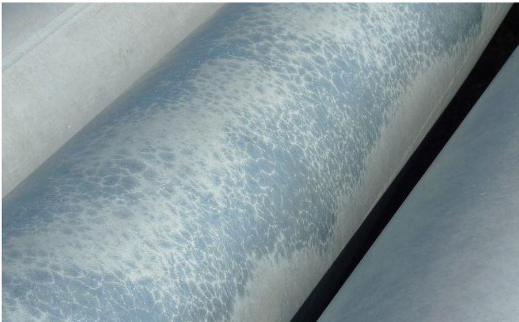
**Figure 3:** This galvanized pipe's steel composition is likely to be in Category B, shown by the scale-like appearance of the coating, where some of the Fe/Zn alloy has extended through to the surface. This product complies with AS/NZS 4680. Over time, the surface will change to a more even dull grey finish.
